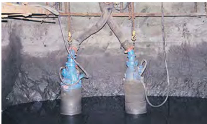
: Slimline Pumps - Pump diameter less than 15"
