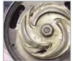
Competitor Impeller is effectively worn out.
